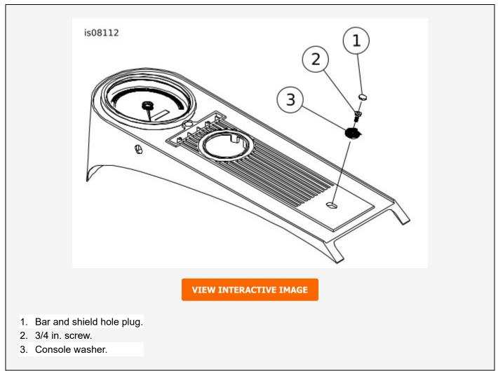
Figure 1. Installation on FLHR Instrument Panel
