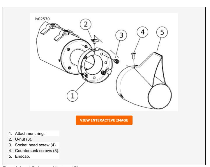
Figure 2. Install Endcap on Attachment Ring
