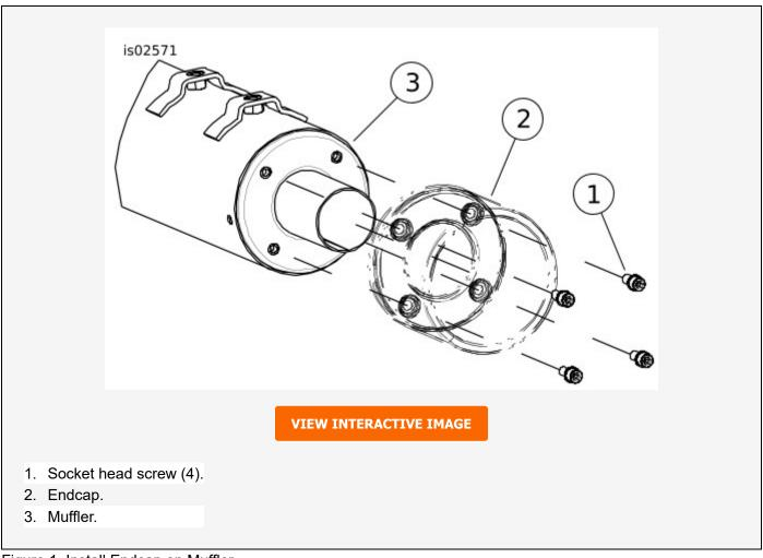
Figure 1. Install Endcap on Muffler
